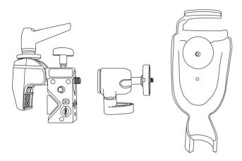
Secure the XL Vu mini magic clamp and place the XL Vu system in the handset holder.
