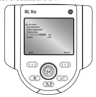
**Note:** Turning on FREEZE FRAME is a convenient way to turn off the light output and is ideal for changing optical tips and conserving battery charge.
