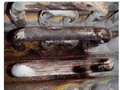
Crude Unit Convection Cross-Over's may suffer severe corrosion due to crude slate changes to higher TAN Crudes
