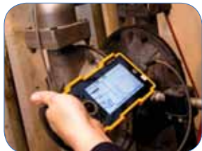
USM Go is an ultra-portable, light-weight pulse-echo flow detector for general purpose testing.
