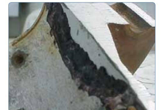
HF scale and corrosion can significantly compromise flange integrity
