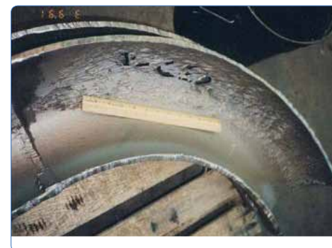
Crude Unit Convection Cross-Over's may suffer severe corrosion due to crude slate changes to higher TAN Crudes
