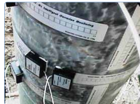
REAC pipe condition can be continuously assessed regardless of process service conditions in typical operation
