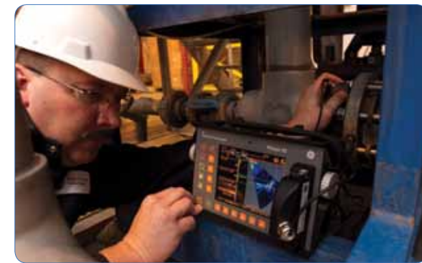
Phasor XS can be applied to the important challenge of detecting and sizing corrosion on flange faces at HF Alky units at oil refinery units.
