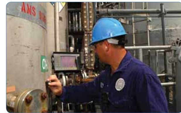
The Phasor CV/DM ultrasonic flaw detector is optimized with software and special dual-element phased array transducers for increased coverage and probability of detection on tank walls, pipes, bolts and flanges.
