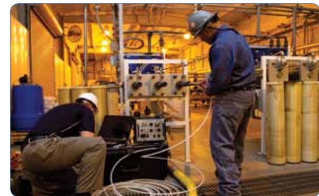
Apollo is a multi channel/multi-frequency digital eddy current instrument, which can drive conventional eddy current testing, remote field as well as large array probes.
