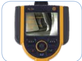
Remote Visual Inspection with Menu Directed Inspection™ for turbine blade viewing.
