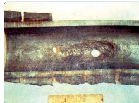
Localized corrosion damage in carbon steel can be confirmed using visual methods
