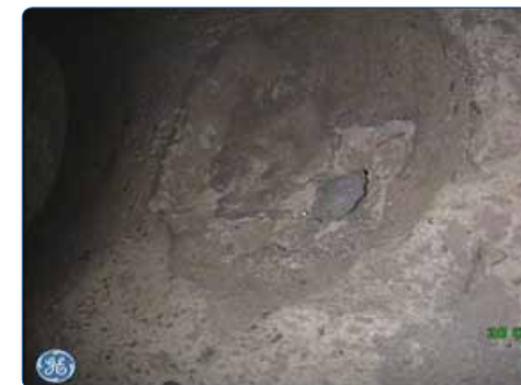
Localized corrosion damage in carbon steel can be confirmed using visual methods
