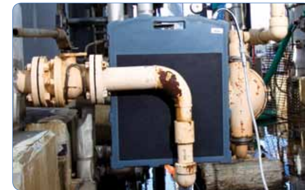
DXR250V is a 16 in x 16 in active area, field-hardened portable imaging digital detector array with a detachable cable. This product plugs directly into a laptop computer for direct radiographic testing and imaging analysis.
