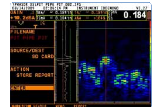
Phasor CV/DM has Dual Element Phased Array capability for accurate, rapid damage sizing
