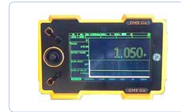
The DMS Go corrosion thickness gage is a simple, easy-to-use instrument for measuring remaining wall thickness of corroded tubes, pipes, tanks and vessels.
