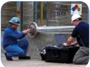
Apollo™ eddy current test instrument performs volumetric interrogation of heat exchanger tube bundle for corrosion and erosion.
