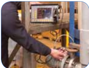
Phasor XS is a proven tool for characterizing safety-critical flange faces at refineries for corrosion and cracking.
