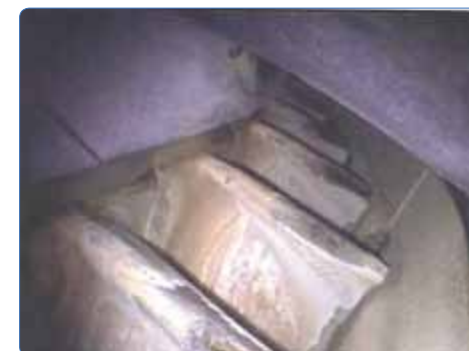
Tip damage (rubbing) can be identified by vibration analysis and monitored off line with RVI
