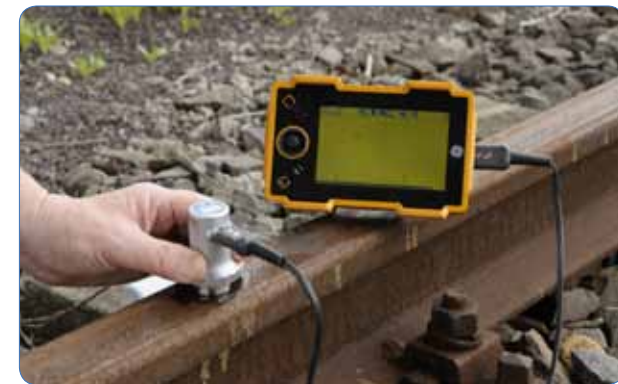
USM Go is an ultra-portable ultrasonic flaw detector weighing only 850 g (1.87 lb). This product has gained wide-spread acceptance for rope-access applications.
