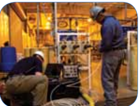
Apollo is a multi-channel, multi-frequency eddy current instrument used to locate and size corrosion, erosion and cracking in heat exchanger tubes.
