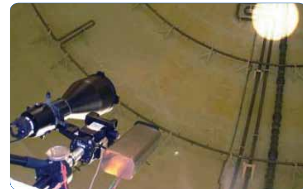
Nuclear plant containment building steel liner is visually inspected with a custom 5-megapixel imaging system to meet ASME's IWE code requirements.
