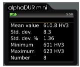
usual for the hardness scale. The Rockwell scales are usually indicated with 1 decimal place, Vickers, Brinell, Shore and tensile strength without any decimal place. The relative standard deviation is displayed with 2 decimal places.
