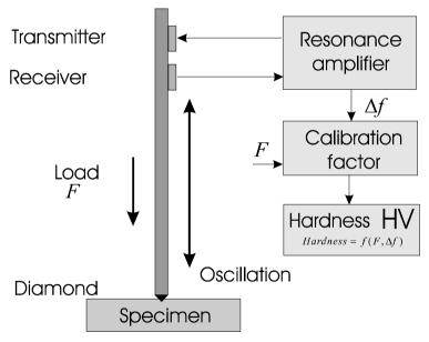
The advantages of the UCI method are the ease of automation and the very good reproducibility of the hardness readings. The reproducibility of the measurements is better than with optical methods of hardness testing because the total area of contact (proportional to d²) enters into the measurement and not only the diagonal d or a diameter. Moreover the measurement results are
