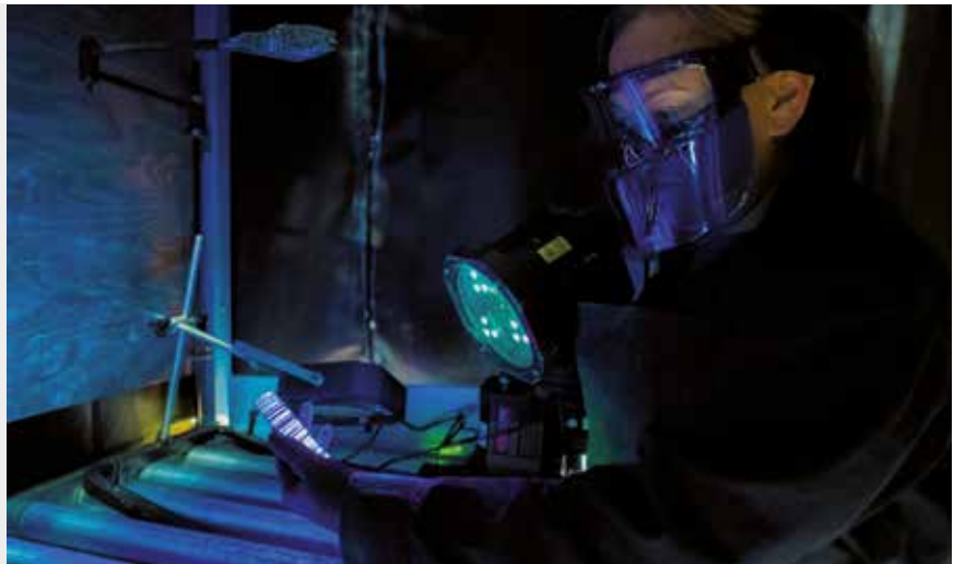
NDI Technician of the 437th Maintenance Squadron checks a cracked chrome panel from a C-17 with a Labino BB 2.0 Series at Joint Base Charleston, S.C.
