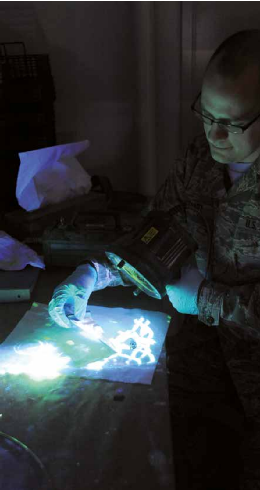
NDI Technician of the 180th Fighter Wing, uses a Labino BB 2.0 Series UV light to inspect an F-16 Fighting Falcon compressor blade for cracks during unit training assembly in Swanton, O.H.
